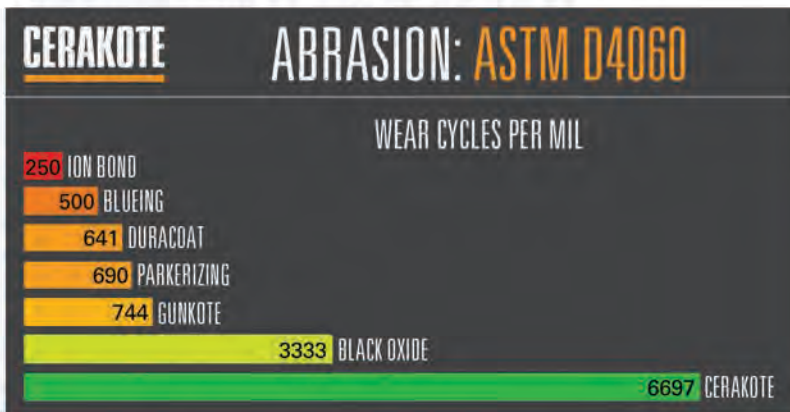
Figure 11. Abrasion testing results demonstrate the coating's capability to substantially increase durability. Visit http://www.youtube.com/user/nictraining for the full video.
