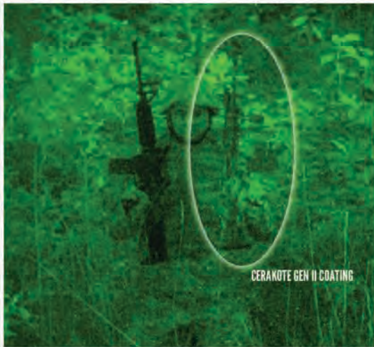
Figure 3. N-IR signature is managed by emulating the background reflectivity. The weapons on the right and top are coated with one of the products offered in the Cerakote™ Gen II line.
